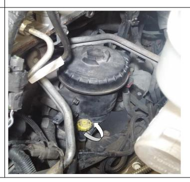
3. Disconnect the fuel heater and WIF sensor connectors.
