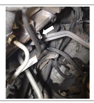
9. Remove the three (3) screws holding the bracket to the engine using a 10mm socket.
