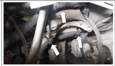
7. Remove the return quick-connect and remove the banjo bolts from the fuel return bracket with a 17mm socket. Set these aside, as they will be re-used later for install.
