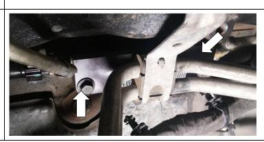
Using the supplied insulated loop clamp, and bolt. Secure the starter cables to the top of the motor mount.
