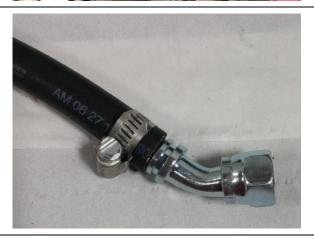
21. Ensure all fittings are tight, and hoses are zip tied away from any hot or moving parts in the engine bay.
