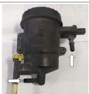
5. Remove the bolts holding the fuel bowl and filter assembly using a 10mm socket, and remove the bowl from the engine bay.
